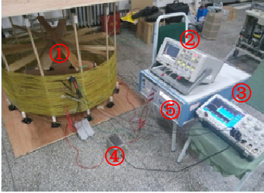
Fig. 2. Experimental schematic diagram.(① experimental winding, ②③ oscilloscope, ④ Pearson broadband current sensor shielded by box ⑤ surge generator)
